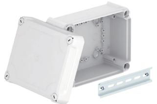
Closed junction box for the connection of cables and lines indoors and in protected outdoor areas. Rectangular design without entries. Suitable for wall and ceiling mounting and on mounting panels. With the option to fasten inside and to mount via the corner domes. High, transparent cover with quick lock, sealable. Made from halogen-free materials.
