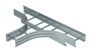
Horizontal T branch piece, for all wide span cable ladders of 160 mm side height. For further stabilisation, additional supports should be planned for the area of the fittings.
