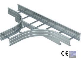
Horizontal T branch piece, for all wide span cable ladders of 160 mm side height. For further stabilisation, additional supports should be planned for the area of the fittings.
