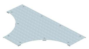
Cover for wide span T branch piece with pre-mounted turn buckles. As the connector is mounted from the outside, the fitting cover is 300 mm shorter than the corresponding fitting. This must be considered when installing the track elements.
