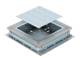
Underfloor accessory box for screed-covered underfloor installation ducts with sheet steel side walls. To mount installation units of the selected nominal size. Height can be infinitely adjusted to the nominal screed height (rapid adjustment possible) and the screed can be worked flush to the screed scraping edge. With noise decoupling option after screed laying and can be used with system accessories, also for heavy-duty application.
