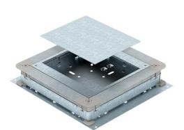
Underfloor accessory box for screed-covered underfloor installation ducts with sheet steel side walls. To mount installation units of the selected nominal size. Height can be infinitely adjusted to the nominal screed height (rapid adjustment possible) and the screed can be worked flush to the screed scraping edge. With noise decoupling option after screed laying and can be used with system accessories, also for heavy-duty application.
