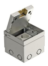
Square floor socket with floor covering recess for use in dry-care cavity and screed floors in indoor areas. Installation housing with pre-marked insertion openings for pipes (M25). Cover adjustable to top edge of floor covering using four height-adjustment supports. The minimum installation depth is 110 mm, the height-adjustment range + 20 mm.
