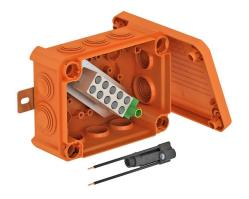
Halogen-free junction box with pre-mounted, soft plug-in seals, approved for the maintenance of electrical functionality according to DIN 4102 Part 12. Maintenance of electrical functionality classes E30 to E90.
