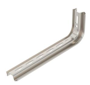
TP support / bracket for the fastening to horizontal concrete ceilings and walls. If the profile is fastened directly to the ceiling or the profile is screwed together as head reinforcement, then, for reasons of stability, always use the spacer, type DS 4.
