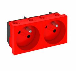
Socket with earthing pin Double 33°, with increased touch protection, with screwless terminals, 2-pin, 16 A, 250V  $\sim$ , with connection terminals to IEC 60884-1.
