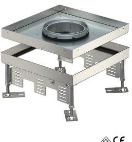
Heavy-duty square cassette for tube body of nominal size 9 for the installation of accessories in trunking systems, raised or cavity floors, in dry or wet-cleaned floors for indoor use. Load class 1 to 10 kN.
