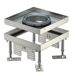
Heavy-duty square cassette for tube body of nominal size 4 for the installation of accessories in trunking systems, raised or cavity floors, in dry or wet-cleaned floors for indoor use. Load class 1 to 10 kN.
