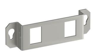
Mounting support to accept two data connection modules of the following types: Brand-Rex: shielded; EKU: E-Stone; Dätwyler: KS-T, MS-K and KU-T module; R&M: Snap-In and Keystone; Rutenbeck: UM and UMflex; SETEC: MKJ, UKJ and XKJ; Siemon TERA; Tdegärtner: AMJ and UMJ. Dimensions of a mounting opening in mm: 19.30 x 14.80. Suitable for GE2F installation unit with tube body.
