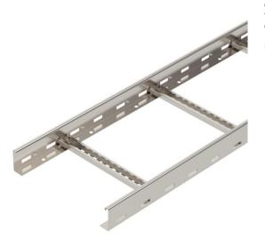
Cable ladder with 60 mm side height with welded C30 profile rungs which are open in an upwards direction. Rolled side rail for reinforcement and as edge protection. Fastening to the bracket takes place using clamps, type LKS 40. The slot dimension of the frame is 16.5 mm and the appropriate clamp clip is type 2056.
