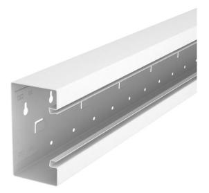
GS device installation trunking for mounting on the wall or on fastening panels. The GS device installation trunking possesses self-contacting locking straps to accept a sheet steel partition. The equipotential bonding between the trunking bases takes place using the trunking coupling. The protective measure and the equipotential bonding is guaranteed between the cover and the base by the selfcontacting trunking cover. The real system opening is 76.5 mm. The cover must be ordered separately.
