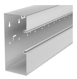
GS device installation trunking for mounting on the wall or on fastening panels. The GS device installation trunking possesses self-contacting locking straps to accept a sheet steel partition. The equipotential bonding between the trunking bases takes place using the trunking coupler. The protective measure and the equipotential bonding is guaranteed between the cover and the base by the self-contacting trunking cover. The real system opening is 76.5 mm. The cover must be ordered separately.
