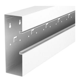
GS device installation trunking for mounting on the wall or on fastening panels. The GS device installation trunking possesses self-contacting locking straps to accept a sheet steel partition. The equipotential bonding between the trunking bases takes place using the trunking coupler. The protective measure and the equipotential bonding is guaranteed between the cover and the base by the self-contacting trunking cover. The real system opening is 76.5 mm. The cover must be ordered separately.
