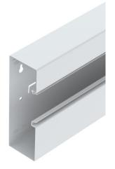
GS device installation trunking for mounting on the wall or on fastening panels. The GS device installation trunking possesses self-contacting locking straps to accept a sheet steel partition. The equipotential bonding between the trunking bases takes place using the trunking coupler. The protective measure and the equipotential bonding is guaranteed between the cover and the base by the self-contacting trunking cover. The real system opening is 76.5 mm. The cover must be ordered separately.
