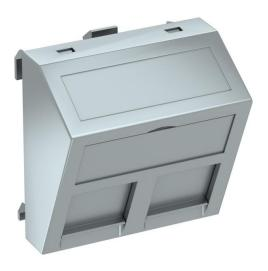
Data technology support with slanting outlet and locking slider to accept two data technology connection modules with RJ45 socket. The locking fastening is suitable for horizontal and vertical installation in the system environment. Type RM has a special module seat and is designed for indirect fastening of the data connection modules in the mounting opening.
