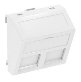
Data technology support with slanting outlet and locking slider to accept two data technology connection modules with RJ45 socket. The locking fastening is suitable for horizontal and vertical installation in the system environment. Type B has a mounting opening of  $19.35/21.55 \times 14.85 \, \text{mm}$  and is designed for direct fastening of the data connection modules in the mounting opening.
