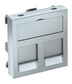
Data technology support with straight outlet and locking slider to accept two data technology connection modules with RJ45 socket. The locking fastening is suitable for horizontal and vertical installation in the system environment. Type RM has a special module seat and is designed for indirect fastening of the data connection modules in the mounting opening.
