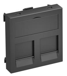
Data technology support with straight outlet and locking slider to accept two data technology connection modules with RJ45 socket. The locking fastening is suitable for horizontal and vertical installation in the system environment. Type C has a mounting opening of  $19.30 \times 14.80$  mm and is designed for direct fastening of the data connection modules in the mounting opening.
