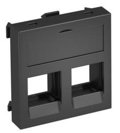
Data technology support with straight outlet and without a locking slider to accept two data technology connection modules with RJ45 socket. The locking fastening is suitable for horizontal and vertical installation in the system environment. Type C has a mounting opening of 19.30 x 14.80 mm and is designed for direct fastening of the data connection modules in the mounting opening.
