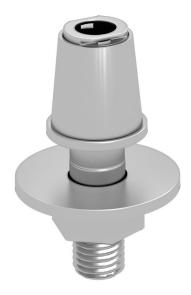
Stainless steel fastening stand for fixed mounting of a Deskbox type DB-... on a tabletop. It is mounted using a drill hole (Ø16 mm) in the tabletop.
