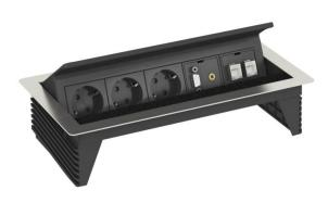
Foldable Deskbox with connection cable for fixed installation in a tabletop, housing made of brushed stainless steel with brush bar as cable outlet. Mounting is done via an installation opening 295 x 157 mm in the tabletop.
