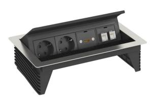
Foldable Deskbox with connection cable for fixed installation in a tabletop, housing made of brushed stainless steel with brush bar as cable outlet. Mounting is done via an installation opening  $245 \times 157$  mm in the tabletop.
