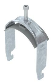
Clamp clip with U-foot, plastic pressure sleeve made of polypropylene. For vertical and horizontal mounting of 1 single cable on a C-profile rail. For slot width 18–22 mm. With 1-start screw thread on pressure sleeve, universal hexagonal screw head WAF10, with slot and cross recess. Suitable for assembly indoors and outdoors. We recommend the use of a counter-sleeve.
