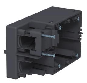
Installation trunking box for installation of a CEE socket with four-point fixing track 60 x 60 mm or 70 x 70 mm; with external strain relief for jacketed cables of up to  $\emptyset$  18 mm; with eccentric lock for quick, screwless fixing.
