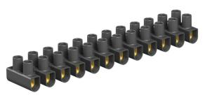
Tested to EN 60998. Steel terminals, steel screws, electrogalvanised, 12-pole, individual terminals detachable from strips using "twist'n'pull". Captive upwards screw. Max. approved ambient temperature to EN 60998: -5 to +80 °C. Nominal cross-section 10 ÷ mm<sup>2</sup>. Nominal voltage 450 V. Nominal current 57 A. Max. attachment each side: 10 mm<sup>2</sup> single-wire or 6 mm<sup>2</sup> multi-wire/flexible.
