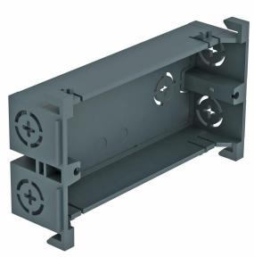
Front-locking, double device installation socket for British Standard switch systems. Insertion opening for cable diameters of max. 17 mm. Can be used in all device installation trunking of the Rapid 80 series and ISS service poles with 76.5 mm system opening.
