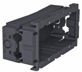
Front locking accessory mounting box for standard switch ranges for the installation of two individual installation devices or a multiple protective contact socket. With unfolding, and also removable, base for time-saving cable connection and with feed openings for cable diameters of up to 14 mm. Halogen-free version. Vertical fixing track 60 mm.
