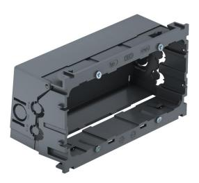
Front locking accessory mounting box for standard switch ranges for the installation of two individual installation devices or a multiple protective contact socket. With unfolding, and also removable, base for time-saving cable connection and with feed openings for cable diameters of up to 14 mm. Halogen-free version. Vertical fastening track 60 mm.
